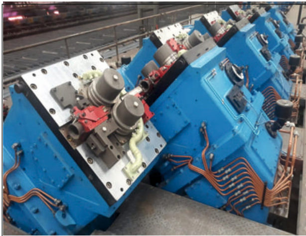
100 mps Wire Rod Block Designed by KOBELCO Japan successfully Commissioned at Madhav Alloys
