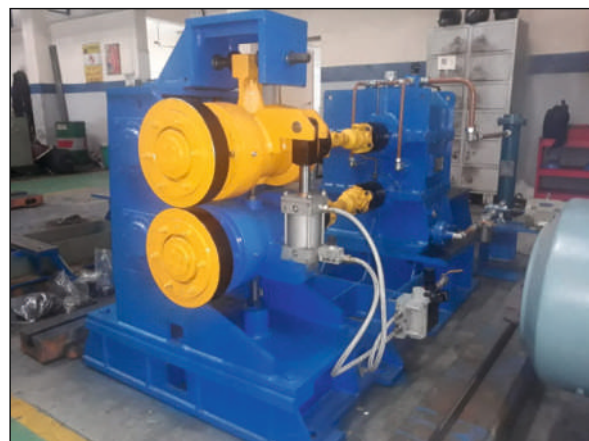
High Speed Pinch Roll @ 30 mps
